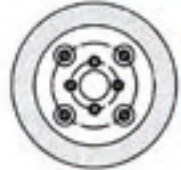
23ST11 internal bolting
